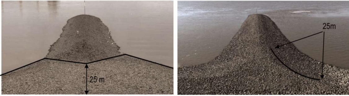
Figure 2 Groyne Geometries Used in the Prototype Experiment. Left: B29 with Recessed Root Area. Right: B31 with Reinforced Root by Broadened and Rounded Transition Area to the Bank Revetment
