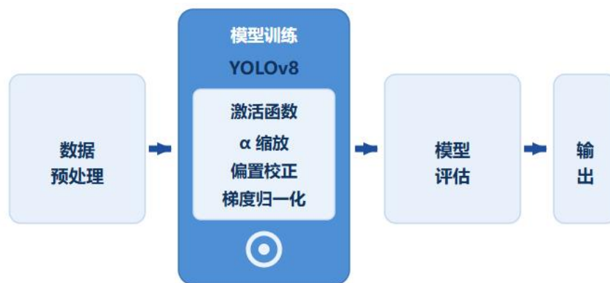
Figure 1 Conceptual Framework of the Modified YOLOv8m Model for Vehicle Classification
